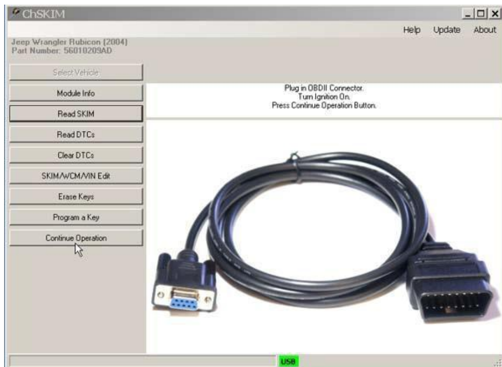
Figure 19. The SKIM number reading via OBD II
