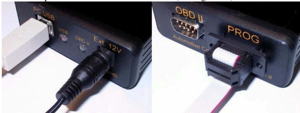
Figure 11. Required connections for the In-circuit EEPROM programming
