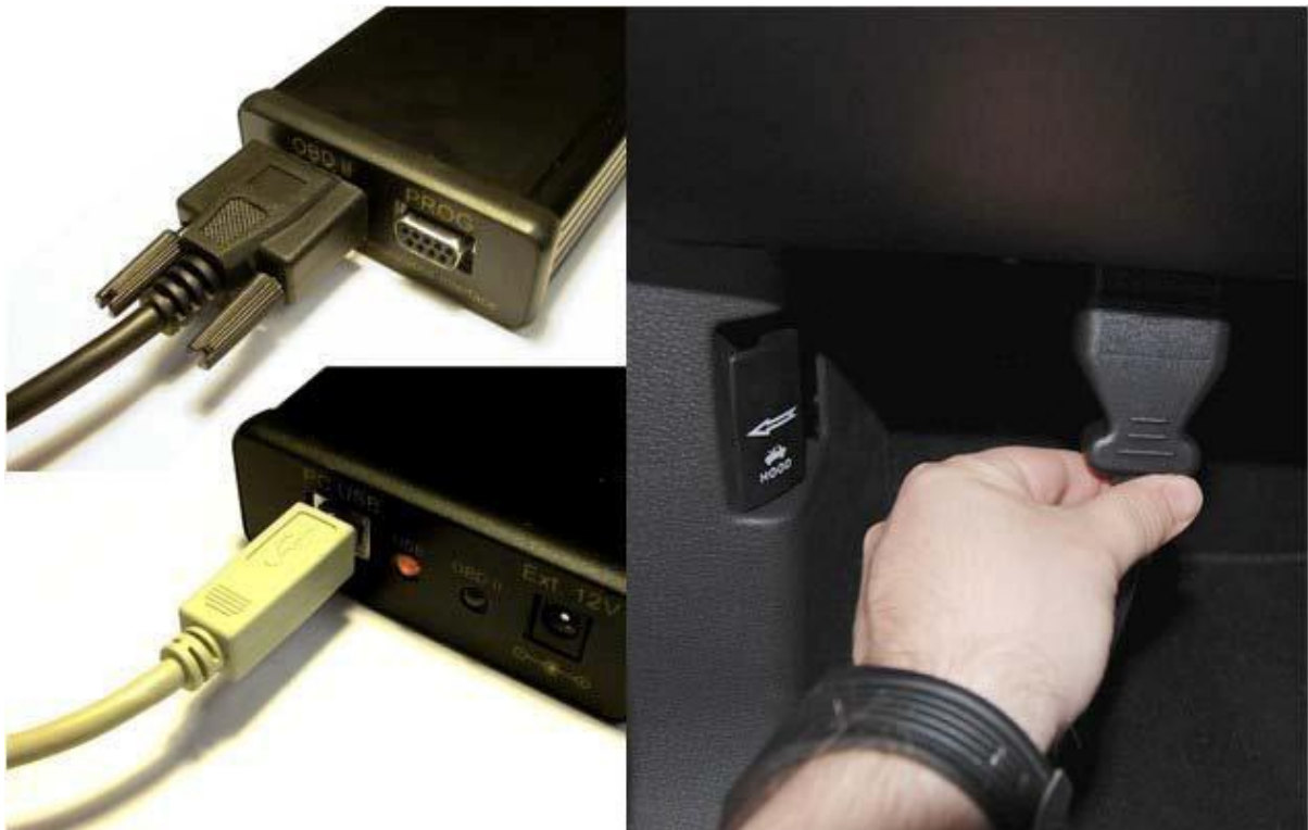
Figure 17. Connection of DMAX-Tool to vehicle
