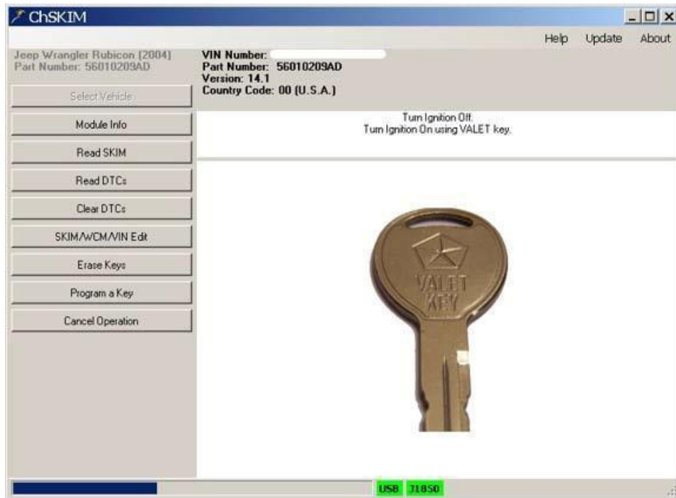
Figure 22. The SKIM number reading, step 3 Turn the ignition off.
