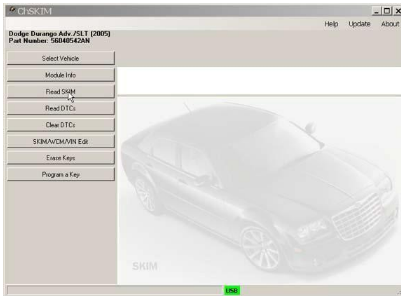
Figure 24. The SKIM number reading via OBD II-CAN
