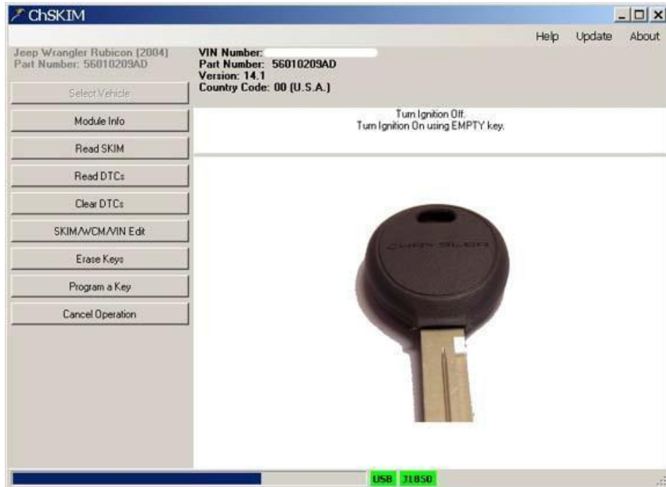
Figure 22. The SKIM number reading, step 3
