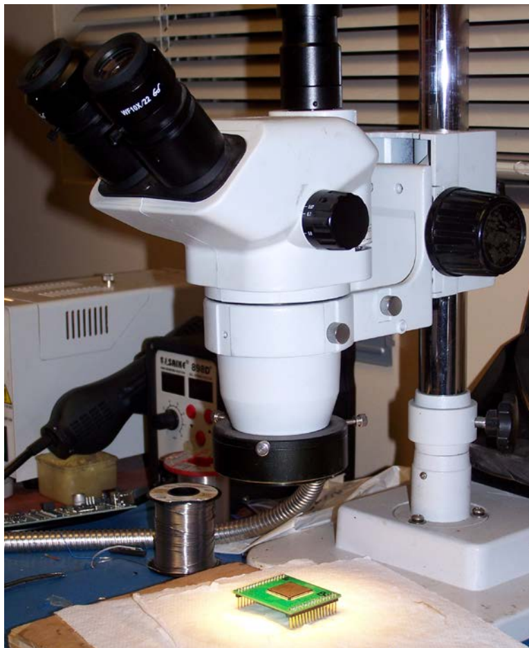
Figure 19 Using Inspection Microscope to control soldering quality
